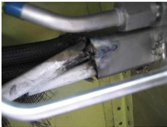
The complete system and related components were inspected. A short was present with the starter/generator cables. The left pylon lower panels were removed and the area inspected. A short was discovered at the pylon feed through cable support as shown in the photo to the left.
